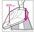
Line up edge of Pad with PAD EDGE INDICATOR LINE. Gently place unit on Ultramicrofiber pad. You are now ready to steam clean.
